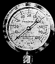
Steam Pressure Gauge.
